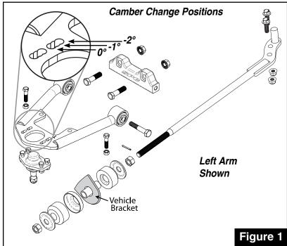
ring is sitting within body mount. Torque caster rod to lower control arm bolts to 90 ft-lb [122 Nm].
