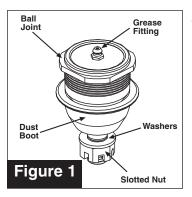
to Mustang II independent front suspension systems, the ball joint comes complete with the necessary spacer to adapt it to the Mustang II spindle. This ball joint is a flat top style which accepts the decorative stainless steel end caps used in many Street Rod applications.
