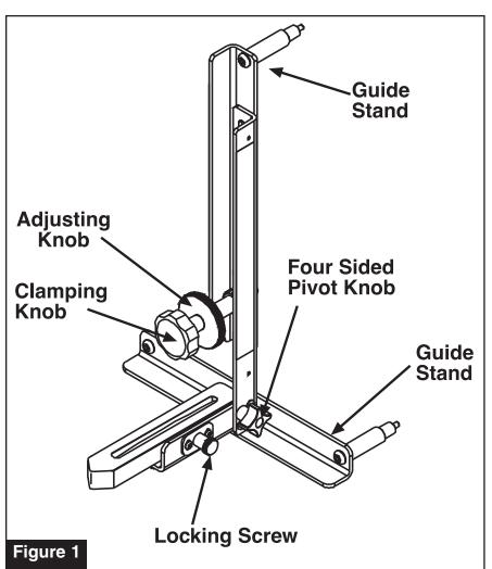
pressure for a snug fit and tighten the black clamping knob. In cases that the wheel has no rim or lip to grasp, simply hold the tool to the accessible flat surfaces and read your camber angles or changes.
