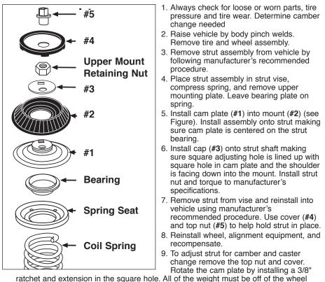
and the suspension must be hanging before rotating cam plate.
