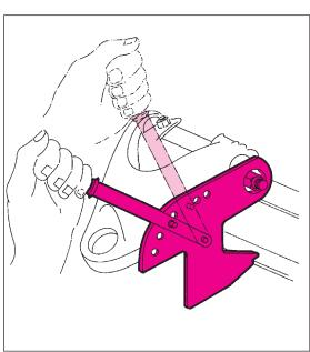
5. After adjustment is made, tighten bolts to manufacturer's specifications.
