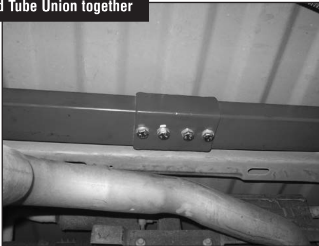
Figure 2 Loosely bolt Cross Tubes and Tube Union together
