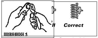
5. For easy installation spread hooks on stabilizer slightly with pliers (see **Illustration 3**).
