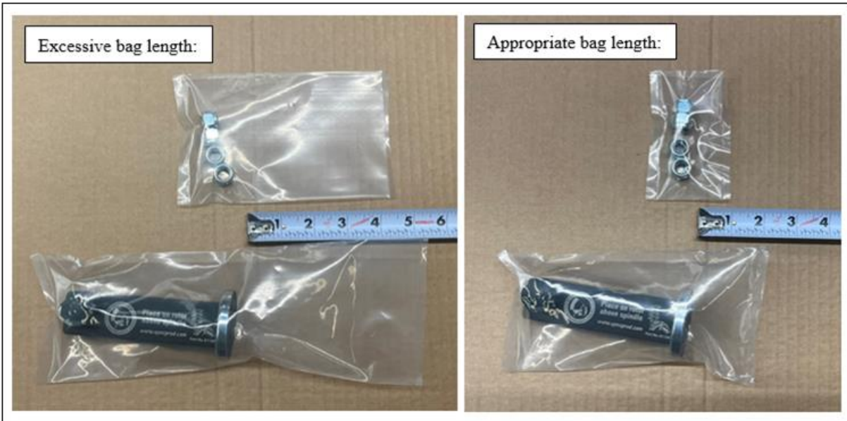
Figure 3: Examples of Excessive and Appropriate Heat Seal Bag Lengths
