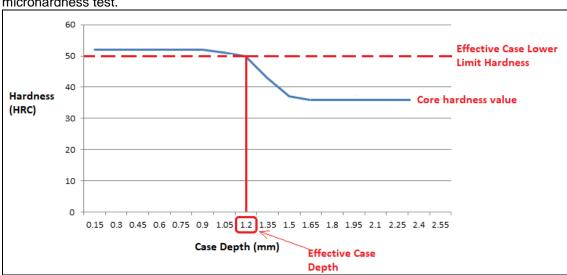
2. Total Case Depth – depth of case from surface to core hardness of part.
